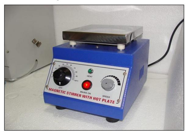
A Magnetic Stirrer with Hot Plate is a laboratory instrument that combines heating and stirring to mix solutions efficiently. It is commonly used in chemical, pharmaceutical, biological, and research laboratories for uniform heating and mixing of liquids.
