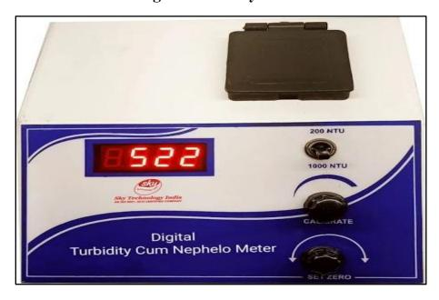
A digital turbidimeter is an electronic device used to measure the turbidity (cloudiness or haziness) of a liquid caused by suspended particles. It works by passing a light beam through the sample and detecting the amount of scattered or absorbed light. The turbidity is typically measured in Nephelometric Turbidity Units (NTU) or Formazin Nephelometric Units (FNU).
