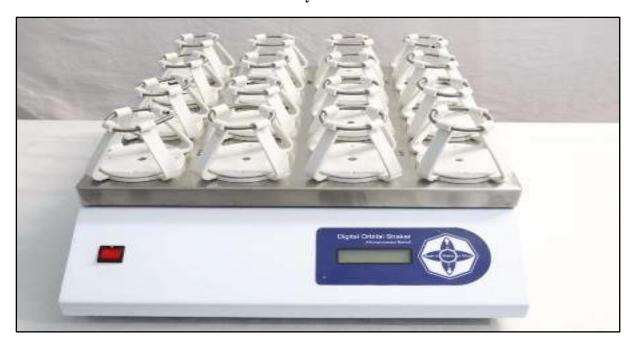
A Rotary Shaker is a laboratory apparatus used to mix, agitate, or stir liquids in test tubes, flasks, or bottles by providing continuous circular motion. It is commonly used in biological, chemical, and pharmaceutical laboratories for sample preparation and incubation.
