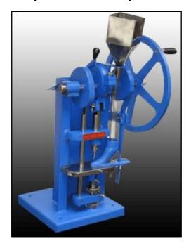
A Hand-Operated Tablet Compression Machine is a manual device used in small-scale laboratories or research settings to produce tablets for experimental or developmental purposes. It is commonly used in pharmaceutical, nutraceutical, and chemical industries for formulation development and testing.
