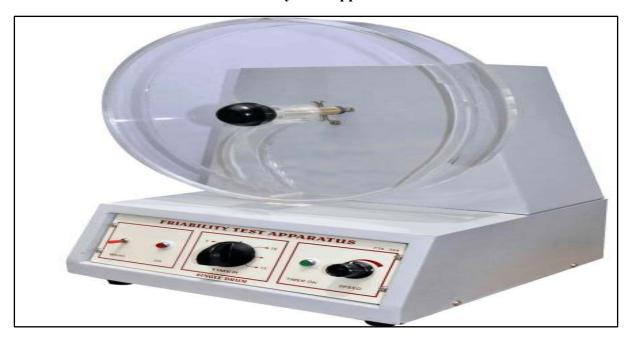
A Friability Test Apparatus is a laboratory instrument used in the pharmaceutical industry to measure the friability (tendency to crumble or break) of tablets during handling, packaging, and transportation. It evaluates the mechanical strength of tablets under stress.
