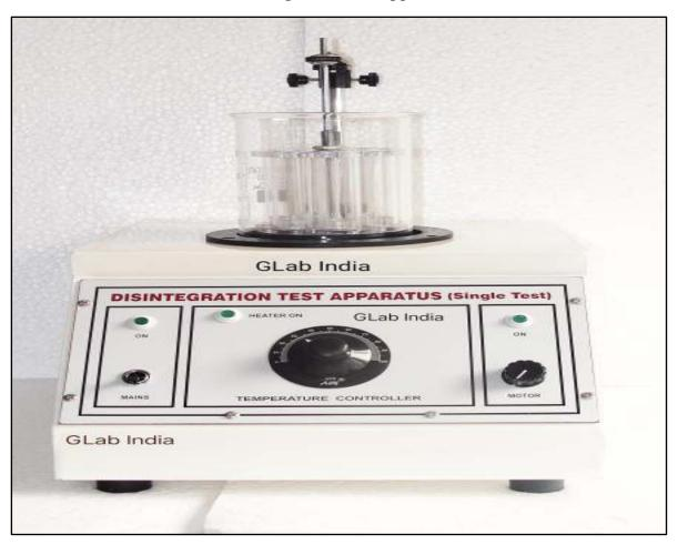
A Disintegration Test Apparatus is a laboratory instrument used in the pharmaceutical industry to evaluate how quickly a solid dosage form (such as tablets or capsules) breaks down into smaller particles or dissolves in a specified medium under controlled conditions. This test ensures that the dosage form meets regulatory standards for dissolution and bioavailability.
