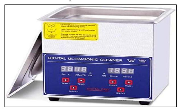
A Digital Ultrasonic Cleaner is a device used for deep cleaning delicate objects using ultrasonic waves and a cleaning solution. It is commonly used in laboratories, medical fields, jewelry cleaning, and industrial applications.
