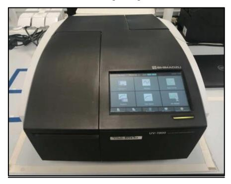
A UV-Vis (Ultraviolet-Visible) Spectrophotometer is an analytical instrument used to measure the absorbance or transmittance of light in the ultraviolet (UV) and visible (Vis) regions of the electromagnetic spectrum (typically 190–900 nm). It is widely used in chemistry, biology, and material science for quantitative and qualitative analysis of substances.
