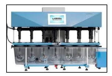
A dissolution test apparatus is a laboratory instrument used to evaluate the rate at which an active pharmaceutical ingredient (API) dissolves from a solid dosage form (e.g., tablets or capsules) in a specified medium. It is an essential tool in pharmaceutical quality control and research to ensure drug consistency, efficacy, and bioavailability.
