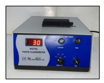
digital photofluorometer is an analytical instrument used to measure the fluorescence intensity of a sample. It is widely used in chemical, biological, and environmental research to detect and quantify fluorescent compounds. Here's a brief overview:
