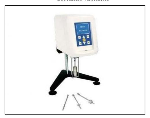
A Brookfield Viscometer is an instrument used to measure the viscosity of liquids and semi-solid materials. It operates based on the principle of rotational viscometry, where the resistance of a fluid to a rotating spindle is measured.
