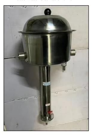
A **steel water distillation unit** is a device used to purify water by heating it to produce steam, which is then condensed back into liquid form, leaving behind impurities. These units are typically constructed from stainless steel for durability and resistance to corrosion. Key features and applications include:
