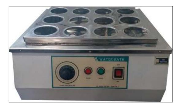
A **rectangular water bath** is a laboratory device used to heat or maintain samples at a constant temperature in a water-filled chamber. It is characterized by its rectangular shape, which provides a larger surface area for holding multiple samples simultaneously. Key features and applications include:
