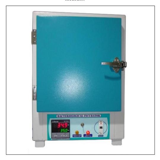
An **incubator** is a laboratory instrument used to maintain a controlled environment for the growth of microbiological cultures, cell cultures, and other biological samples. It provides stable conditions such as **temperature**, **humidity**, **and CO<sub>2</sub> levels** to support optimal growth.
