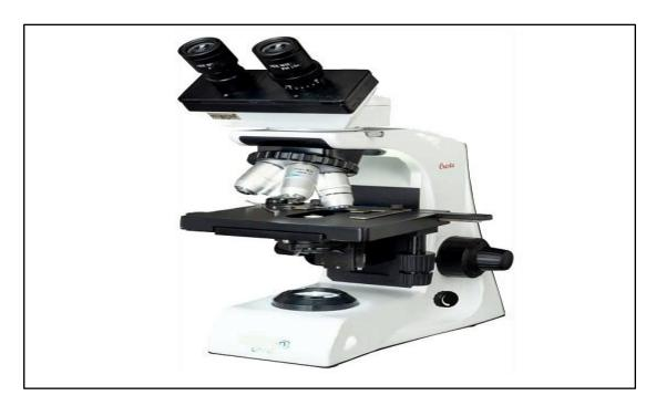
A **binocular microscope** is an optical microscope equipped with two eyepieces (ocular lenses) for viewing samples with both eyes simultaneously. This design reduces eye strain and improves comfort during prolonged use. Key features and applications include:
